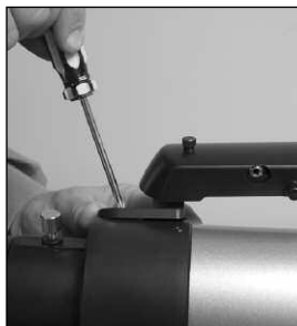
Fig. 8b: Attach Smartfinder to the reflector optical tube assembly.
