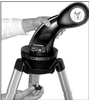
Fig. 5: Attach the mounting arm to the tripod base.
