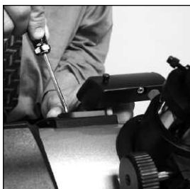
Fig. 8a: Attach Smartfinder to the reflector optical tube assembly.
